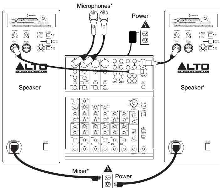
*This diagram is a suggestion for setting up the speaker with audio connections. To pair the speaker with a Bluetooth™ device, see the BLUETOOTH PAIRING & LINKING section below.*
