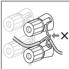
Make sure that exposed speaker wire does not extend outside the speaker terminal and touch any other wire.
