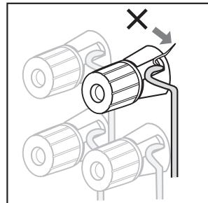
Make sure that exposed speaker wire does not touch the rear panel, screws, etc.
