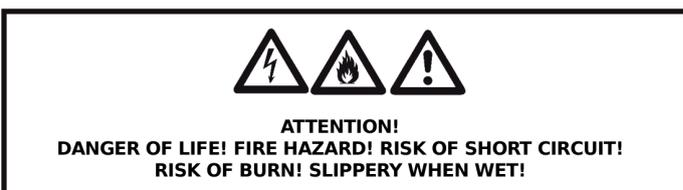
Ensure sufficient ventilation at all times. Insufficient ventilation may lead the fog fluid to condensate, resulting in a slippery surface which may cause accidents. Maintain a minimum distance of approx. 25 cm around the fog machine.
