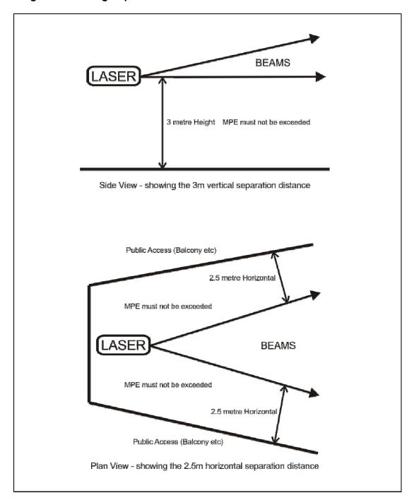
Note. The 3 metre height specified is not the height of the actual projector, but it refers to the height of the laser effect. Therefore having the laser projector positioned at 3m height and aimed directly down is **not** what the guidance is saying.
