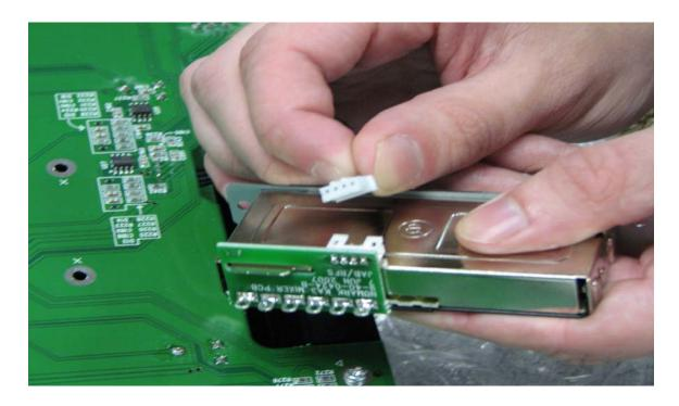
9. Place the crossfader back in the IDJ2 and screw it in securely (3 screws)
