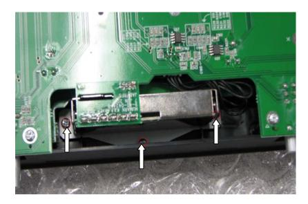
7. Remove crossfader from the IDJ2 and disconnect the white connector.
