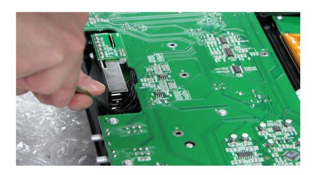
10. Make sure the wires from the crossfader are not sticking out in any way.
