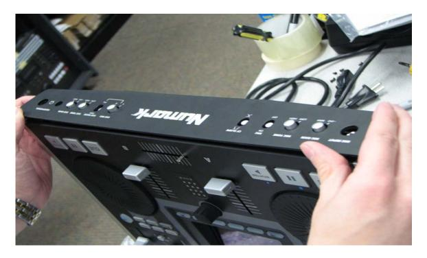
11. Place the back panel back on the IDJ2 and re-attach using the 14 screws from Step 4.
