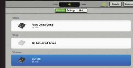
At this point you should now be able to control the DL1608 mixer wirelessly. Also, "CONNECTED" should now be displayed below the Tools icon.
