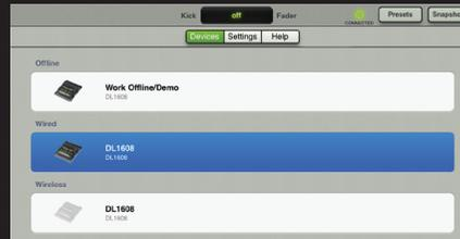
Step 9: There should be three devices listed: Work Offline/Demo, Wired and Wireless. At this point the Wired DL1608 should be selected. Now leave the Tools menu and reconfirm that the DL1608 may be controlled from Master Fader over the wired connection.
