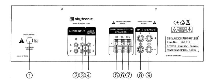
(1) POWER INPUT Power input line (2) A(AUDIO INPUT) A channels signal input jack (3) B(AUDIO INPUT) B channels signal input jack (4) AUDIO OUTPUT Audio signal output jack (5) SR(OUPTUT) Surround right speaker connect pillar (6) SL(OUPTUT) Surround left speaker connect pillar (7) CEN(OUPTUT) Center speaker connect pillar (8) R(OUPTUT) Right speaker connect pillar (9) L(OUPTUT) Left speaker connect pillar
