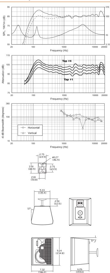
Frequency Response, on axis in half-space  $(2\pi, solid line)$  and full-space  $(4\pi, dotted line)$ , in thru (8 ohm), with Input Impedance
