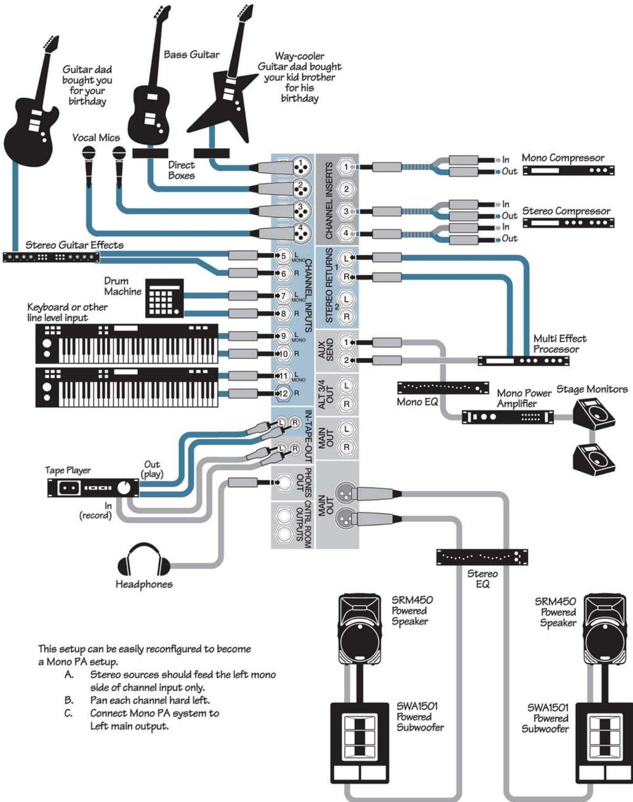
This setup can be easily reconfigured to become a Mono PA setup.
