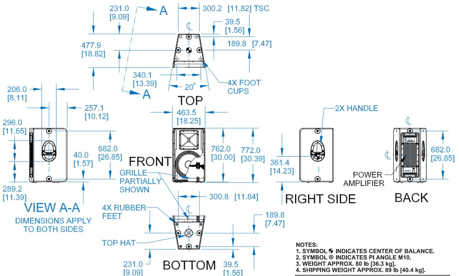
UNLESS OTHERWISE SPECIFIED: ALL DIMENSIONS ARE IN MILLIMETERS. DUAL [INCHES] DIMENSIONS FOR REF ONLY.
