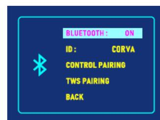
When another speaker of the same model cabinet has the same TWS enabled within Bluetooth range, they will connect as a stereo pair and any Bluetooth audio streamed to the master speaker will be played in stereo across the 2 speakers. (so 2 x CORVA-12A or 2 x CORVA-15A can be a fully wireless stereo pair)
