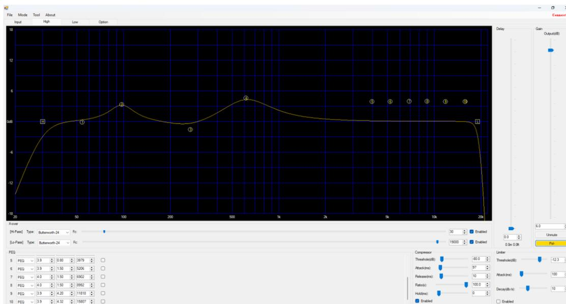
Each driver has **Hi-Pass** and **Lo-Pass** shelving crossover filter sliders directly beneath the frequency graphic. Check the **Enabled** box to activate either crossover, and choose a type from the drop-down list on the left. As with other filters, these can be edited numerically or by dragging the **H** and **L** points on the graph. For woofers the frequency range will most likely be low and for tweeters, the focus will be on high values.
