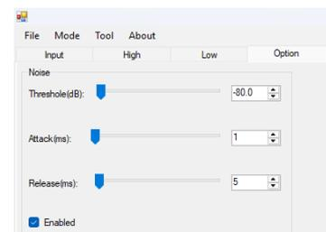
To activate the noise gate, you must check the Enabled box.
