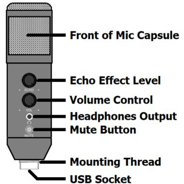
The computer will recognise the CU-POD as a USB Audio Device for both input and output of audio. Connect headphones to the 3.5mm Headphones Output on the front of the CU-POD
