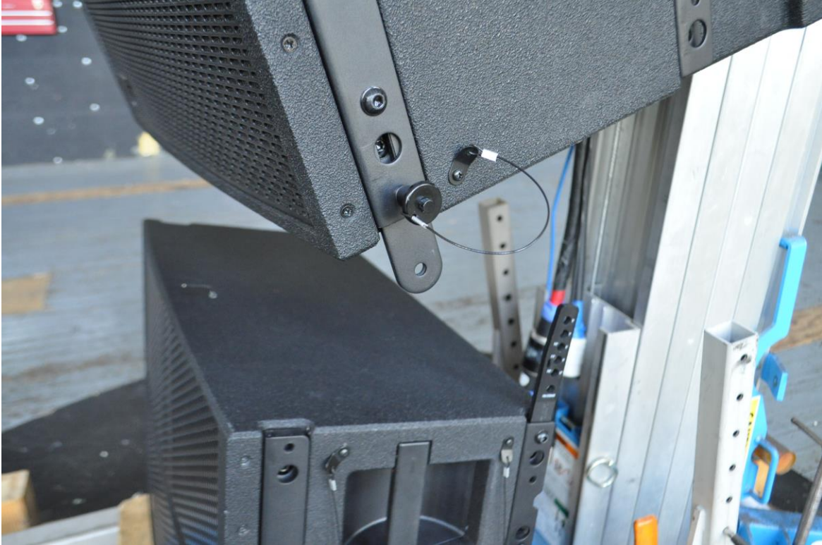
Figure 30 - Rigging tabs pinned into place to allow them to be inserted into the front rigging tube of the lower loudspeaker
