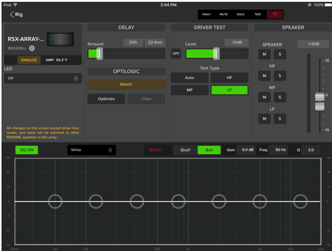
Figure 21 - An array without Optilogic processing assigned
