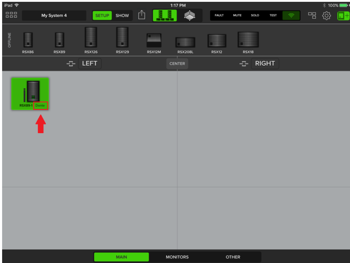
Figure 19 - The RSX89 in EAWmosaic now indicates it has detected a Dante input. This can also be seen on the rear panel of the cabinet itself
