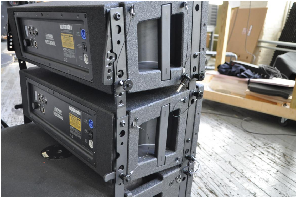
Figure 304 - A RSX208L and RSX12 ground-stacked array
