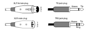
MIC input Connect a balanced microphone to this XLRF input.
