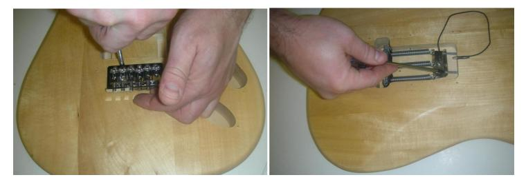
Lie the body face-up on a soft surface. Take the vibrato bridge and sit it into the routed section toward the rear of the body, allowing the sustain block (the metal block underneath the bridge) to hang into the hole through the body.
