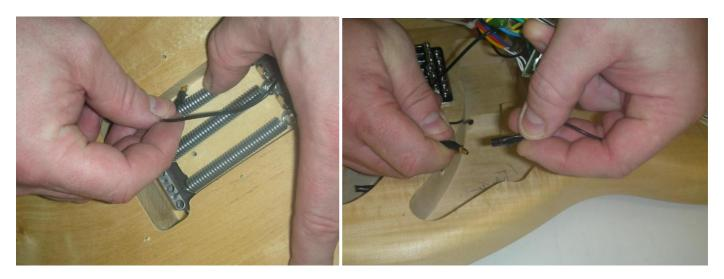
A lead is attached to the spring claw, this should be threaded through the hole halfway along the bottom edge of the rear cavity so that it feeds into the front control cavity.
