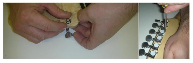
Before attaching the neck to the body, fit the tuning machine-heads to the headstock by inserting the thread through the pre-drilled holes and setting a washer and bush over it.
