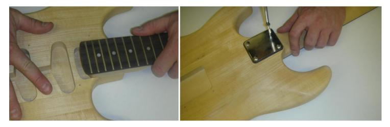
With the body placed on a protective surface face-up, position the neck into the neck pocket until fully inserted.
