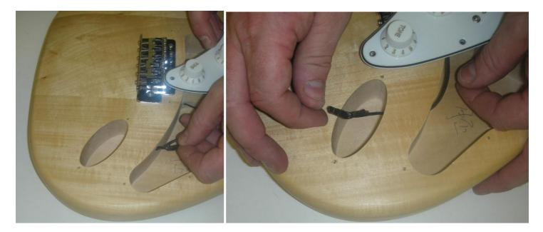
Now position the pick-guard over the front of the body so that pickups and all wiring sit neatly into the routed cavities. Ensure that the edge of the pick-guard sits snugly to the end of the neck and straight to the bridge assembly. Secure the pick-guard with the small dome-head screws provided into the pre-drilled pilot holes.
