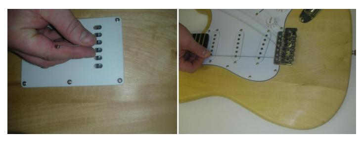
Ensure the string sits smoothly over its saddle and keep taut whilst winding a couple of turns on the relevant tuner. Thread through the string post and bend the string back on itself to anchor it in place. Apply a little tension from the tuner and move on to the next string, repeating the above process for all 6 strings.
