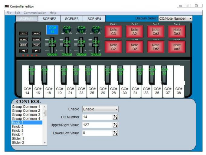
Operating a knob will transmit a control change message. You can enable/disable each knob, specify its control change number, and specify the values transmitted when the knob is turned fully left or fully right..
