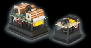
While the drivers are the muscle of a speaker system, the crossover network is the heart and soul. Just one look at a JRX100 network and a competitive network tells the story. JRX100 networks are built using heavy coils with massive cores and heavy gauge wire so they won't saturate when you drive them hard.
