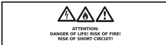
The product must be operated and stored in a dry environment only! Splash water, rain, humidity, fog may reduce the protective insulation which may lead to fatal electric shocks! The limit value for relative humidity is 50% at 45°C. A minimum distance of 1,5 m to a fog machine must be observed; fog saturation in the room must not reduce the visibility to below 10 m.
