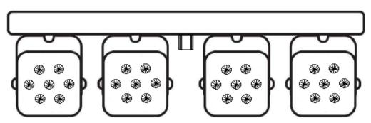
The opened top bar can now be place on to the supplied tripod stand and adjusted to desired height. Each LED PAR Can pans and tilts to face different directions and angles.
