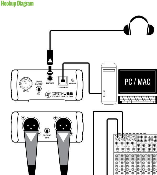
As you can see in this hookup diagram, the MDB-USB is a convenient stereo direct box to add to the chain. Let's look at the front panel connections first. Start by simply connecting a USB cable from the computer's USB slot to the MDB-USB input jack. And end by simply connecting a pair of headphones to the phones I/8" output jack. Front panel connections made!
