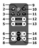
Power on/off 9 Auto 4 sound activated 2 Auto 1 static colours 10 Auto 2 colour change 3 Auto 3 colour fade 11 Auto 5 strobe 4 Static colour -12 Static colour + 5 Program speed -13 Program speed + DMX address -6 14 DMX address + 7 IP slave ID -15 IP slave ID + IP slave mode select 16 DMX mode select
