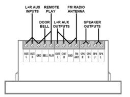
Connect left and right speaker wires to the relevant "+/-" terminals on the WA-215. For better FM reception, an aerial may be connected to the FM ANT and GND terminals.
