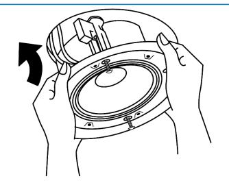
4. Turn the mounting screws in part way to help cut the threads. Install the speaker unit into the cut-out, ensuring that the 4 dog-ear mounts are turned inwards.
