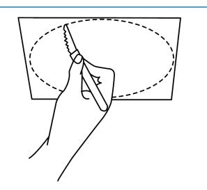
2. Cut out the treed area using a pad saw or other suitable tool.
