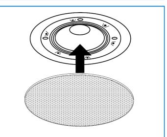
6. Place the speaker grille back onto the speaker, it will fix magnetically.
