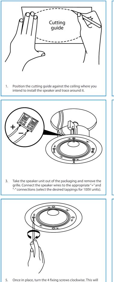
cause the dog-ear clamps to rotate outwards and tighten 6. Place the magnetic magnetic
