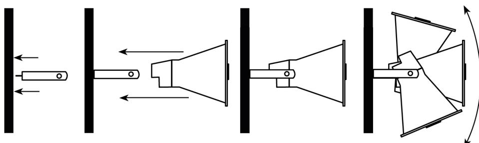
**Warning!** Before installing the speaker, make sure that the wall can hold a minimum point load of 10 times the speaker weight.
