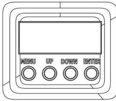
The control board offer several features: you can simple set the starting address, run the pre-programmed program or make a reset. The main menu is accessed by pressing the **Mode**-button, browse through the submenu by pressing **Up** or **Down**.
