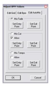
If the 'Allow' for Mix Temp is not checked, the SMART automix will then check if both 'Allow' for Mix Cut are checked. If yes it will do a cut mix (using the cut entry/exit points), otherwise the SMART automix mode will do a standard fade using the Mix Fade entry/exit points.
