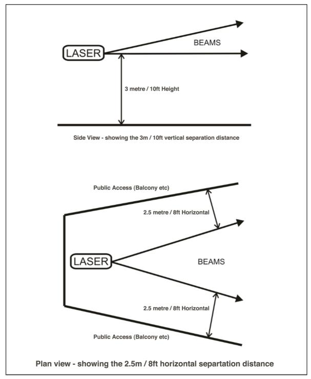
Note. The 3 metre / 10ft height specified is not the height of the actual projector, but it refers to the height of the laser effect. Therefore having the laser projector positioned at 3m / 10ft height and aimed directly down is **not** what the guidance is saying.
