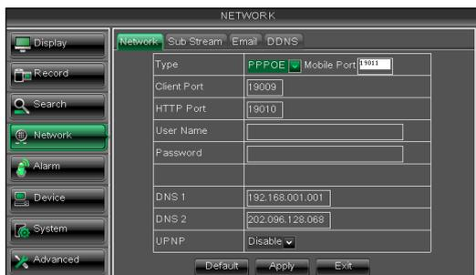
When selecting PPPoE from the Type, user can input user name and password provided by ISP and set Media and HTTP port. And now you can visit your remote DVR by using the IP address captured after registering a domain name and HTTP port and connect to your DVR via public network.
