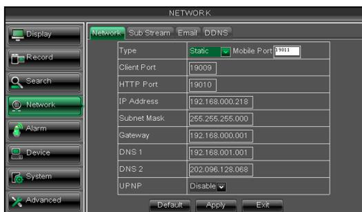
When selecting Static from the Type, user can directly input IP address, Subnet Mask, Gateway and DNS shown as below picture 5-32.
